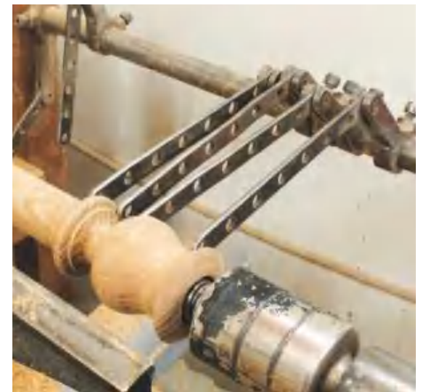
▲ Pic.24 When the first one is finished set the copying fingers up onto the major sizes; this makes the whole turning process much more efficient. Just keep removing wood until the fingers fall off
